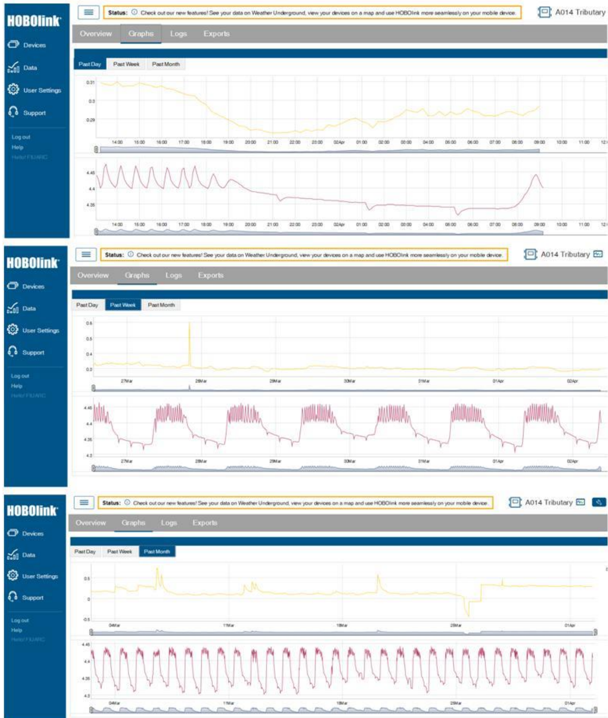
Figure 117. Screenshots of graphs generated in HOBOLink of data collected by Unit 2. Graphs can be generated for recorded data on a daily, weekly or monthly basis.
