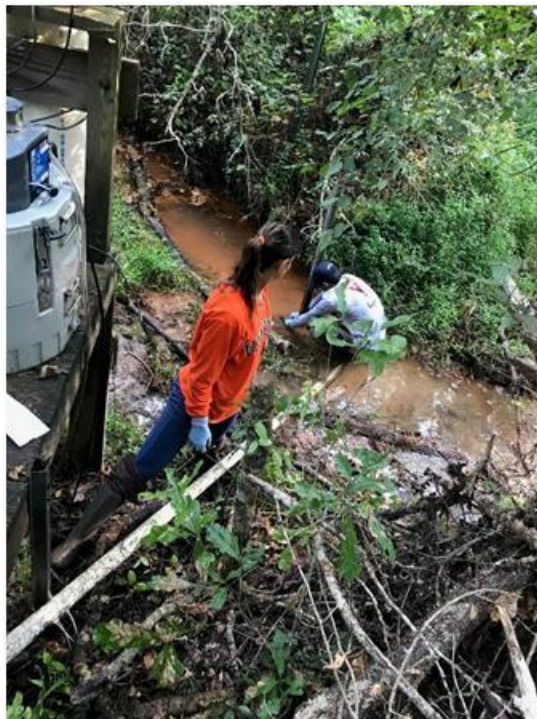
Figure 113. FIU graduate student installing the HOBO RX3000 remote monitoring device in Tims Branch at SRS (left); (right) FIU researcher and student calibrating and testing the device (right).
