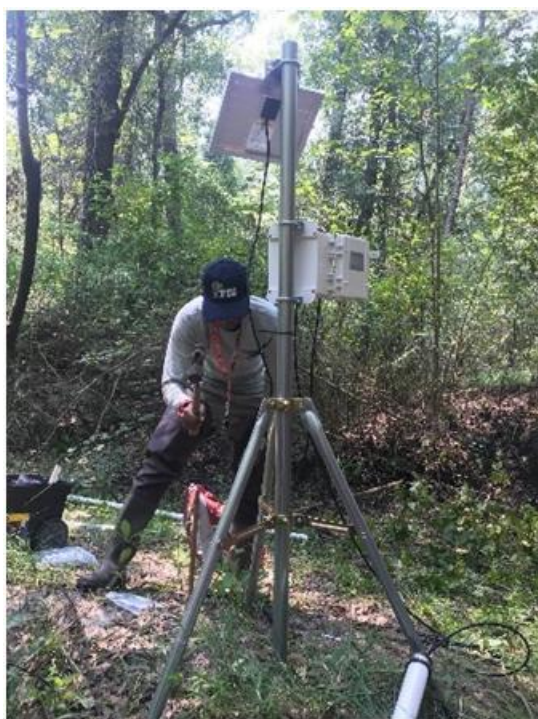
Figure 113. FIU graduate student installing the HOBO RX3000 remote monitoring device in Tims Branch at SRS (left); (right) FIU researcher and student calibrating and testing the device (right).
