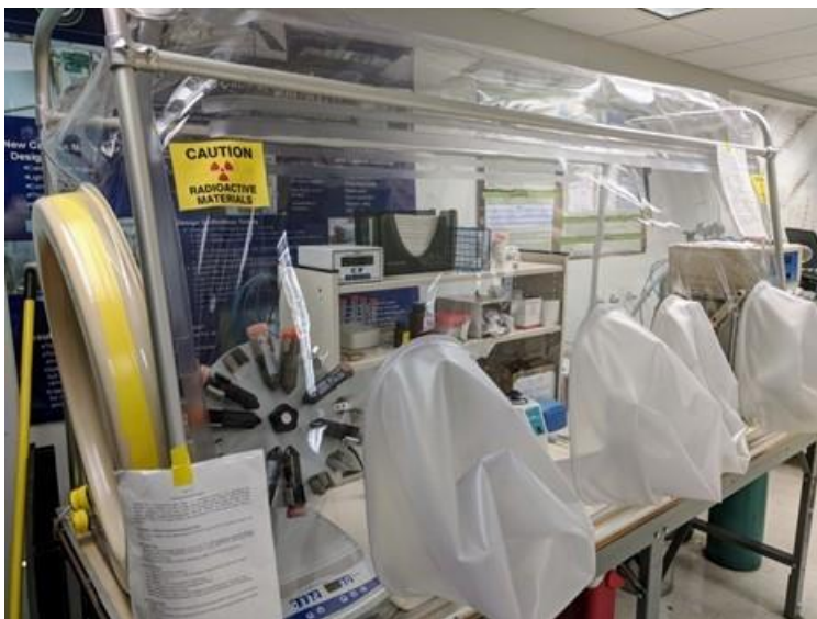
Figure 36. Anaerobic glovebox at FIU EC1227 where pertechnetate reduction experiments are currently taking place under 98% N 2 : 2% H 2 atmosphere.
