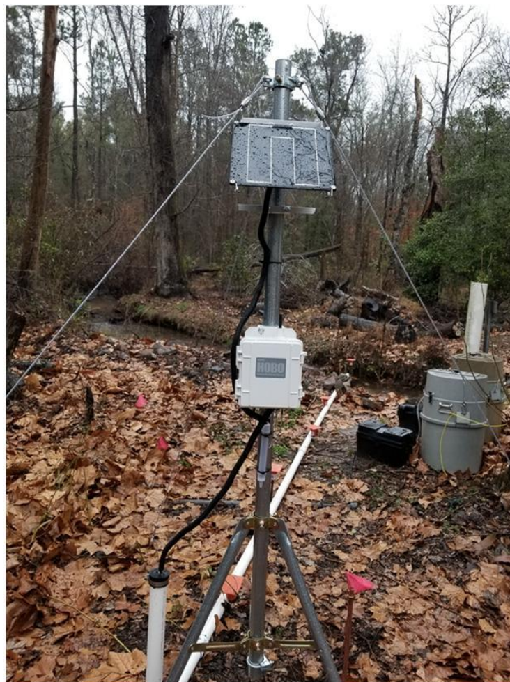
Figure 112. DOE Fellows installing HOBO RX3000 3G Remote Monitoring Stations in the A-014 Outfall tributary and Tims Branch study areas.
