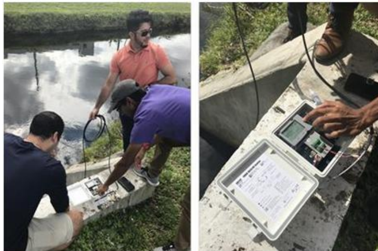
Figure 110. DOE Fellows conducting a field test of the HOBO RX3000 Remote Monitoring System.
